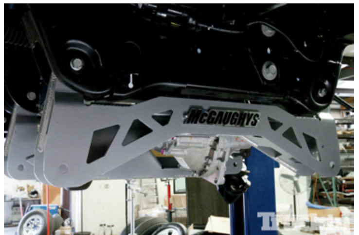
12. The matching front crossmember bolted into the factory control arm sockets with stock hardware. Its arch was designed to maximize ground clearance.
