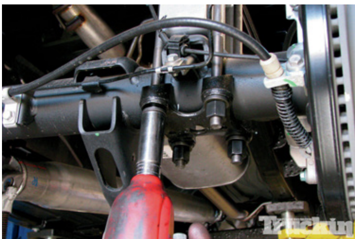
27. Longer U-bolts were used to keep the rear end together using the original cast U-bolt plate that is new for this year.
