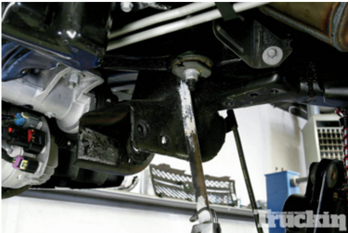
9. This part was not for the faint at heart. The rear control arm crossmember was removed and the mounting ears on the frame were cut back three inches to make room for the beefy McGaughys replacement.
