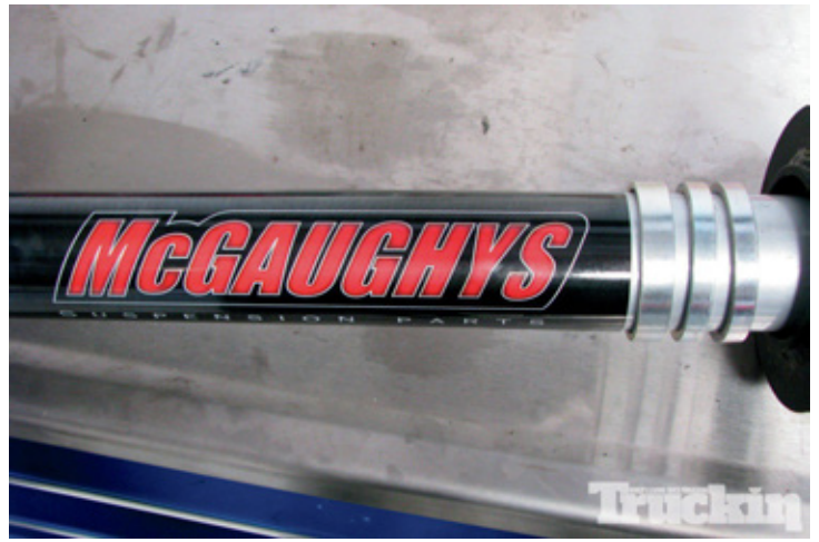
16. One of the optional upgrades we chose was the tuned McGaughys front struts. Combining the McGaughys spring cup, or the original spring cup, with different seat spacers allowed the front suspension height to be altered. We chose eight inches.
