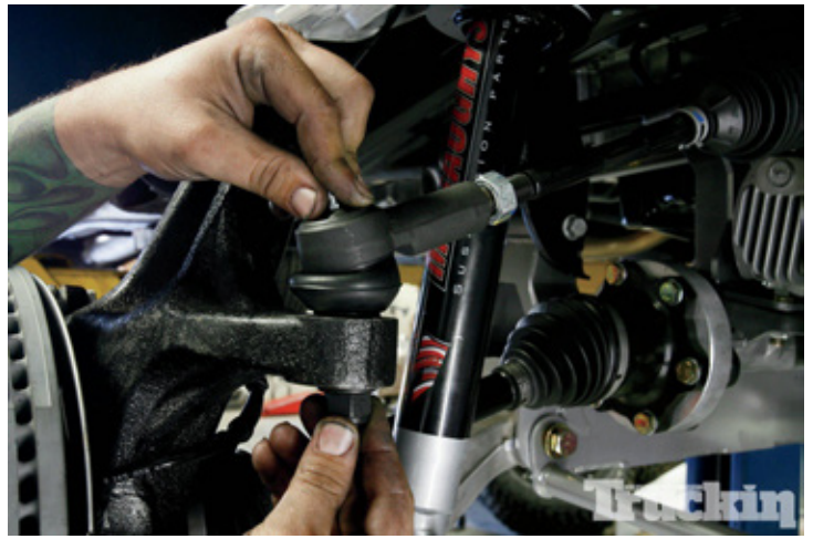
22. Shorter tie rods were supplied in the kit to simplify the swap and remain fully functional with zero steering issues.
