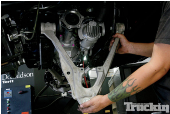
8. We zipped the GMC's lower control arm bolts loose and wiggled the arms off the frame. Thanks to the aluminum construction, they weren't a back breaker to muscle around.
