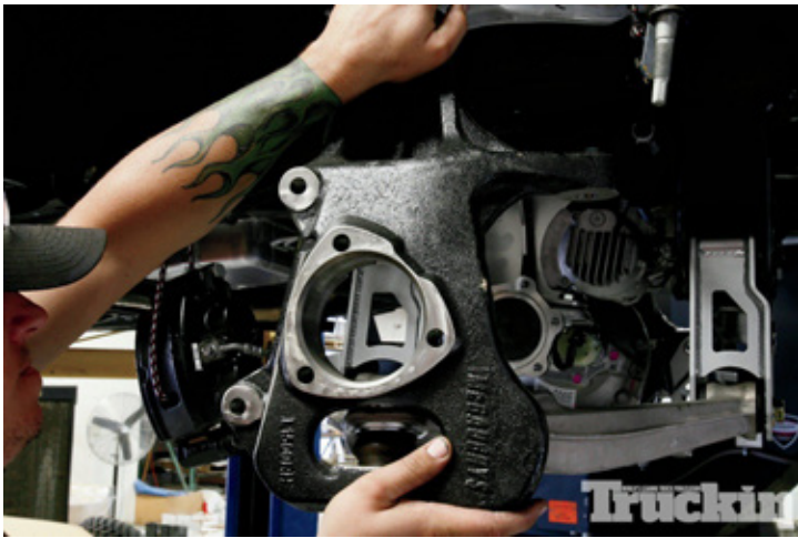
14. McGaughys designed taller spindles to fit its lifted suspension. They are designed to properly pivot a ten-inch wide wheel without scrubbing the tire.
