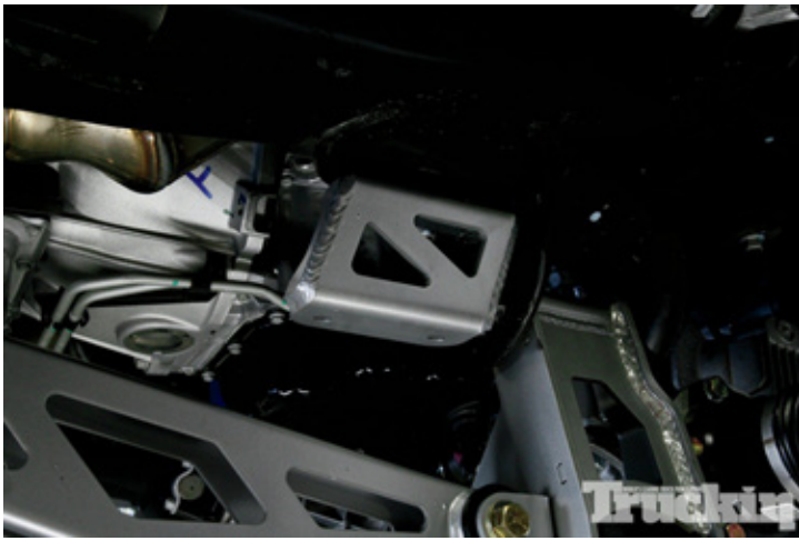
19. Using the original hardware, included spacing brackets were mounted to the frame so the original sway bar could function properly with the lift.
