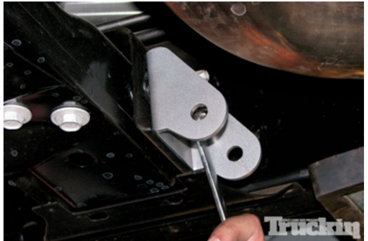
23. To mount the compression struts, the hardware holding the transmission crossmember was loosened. McGaughys designed its rear mounts with slotted holes so that they slipped in place without having to support the transmission.
