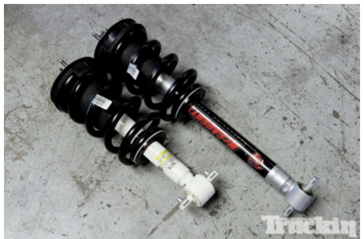
18. Placed side by side, the longer body to accommodate the lift was apparent, but the upgrade in ride characteristics would not be realized until later.
