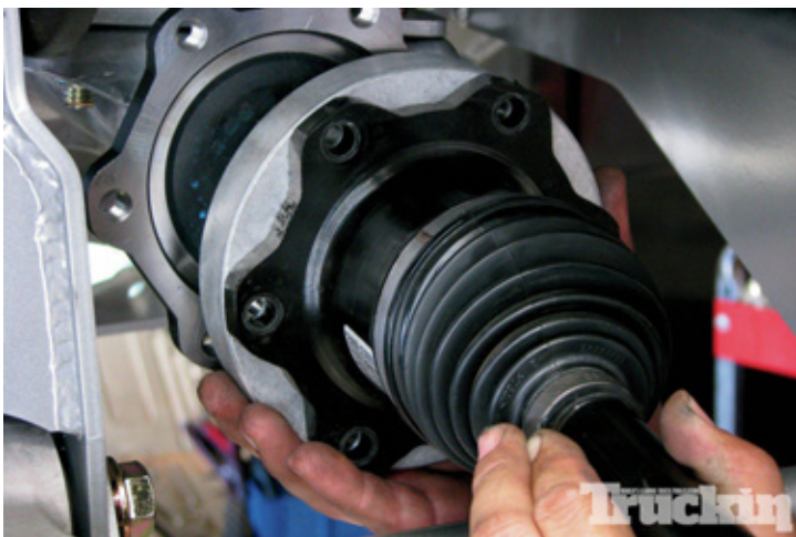
15. Keeping the driveline geometry in proper alignment was the job of aluminum spacers that bolted in behind the front half shafts.
