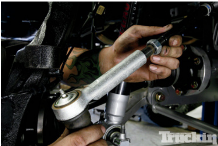
21. To make its new spindles work properly with the electronic power steering and still allow clearance for wider wheels, McGaughys moved the steering arm inward. The original tie-rod ends were too long so they were taken off.
