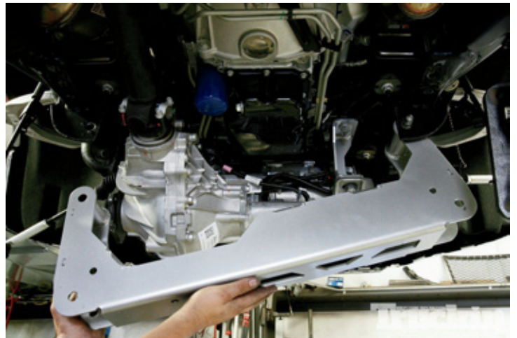
11. As for the rear control arm bracing, the fully boxed replacement was larger and stronger to accommodate not only the lift, but to also address the rigors of off-road driving with oversized tires
