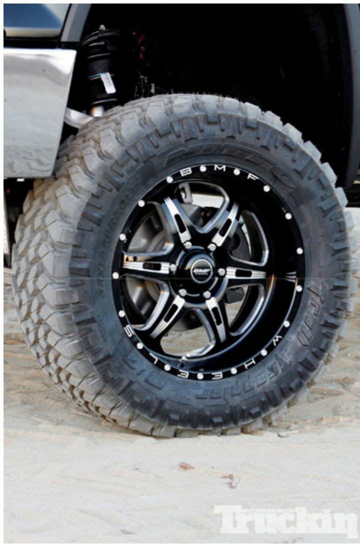
29. With eight total inches of front lift and five inches under the bed, we had great clearance for the 20x9-inch BMF F.I.T.E. wheels encased in burly 35x12.50R20LT Nitto Trail Grappler M/T tires. The new aggressive yet upscale appearance perfectly complements the 2014 Sierras sculpted body lines.
