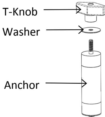
Remove the T-Knob and Washer from each of the Anchor Assemblies.
