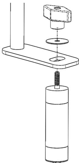
The threads of the Anchor Assembly will fit up into the slots. Replace the Washer and T-Knob. Screw the T-Knob and Washer down until it is finger tight but can still slide freely in the slot.
