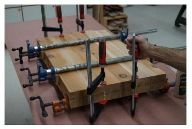
Bridge the seams with clamps, and then close the glue joints with pipe clamps. Make sure the end grain on one end is in perfect alignment. This end will ride against the table saw fence in the next step, so must be straight.
