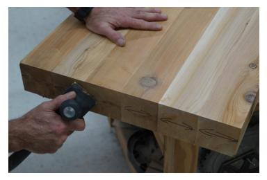
Use a scraper (See Sources) to remove glue residue from the end grain on the table saw fence end of the slab.
