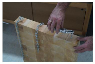
Add hooks and chain. I used 3-3/8" hooks (See Sources) located 2" in from the edge, centered on the thickness of the slab. I chose to hang the target vertically, but you could also hang it horizontally.
