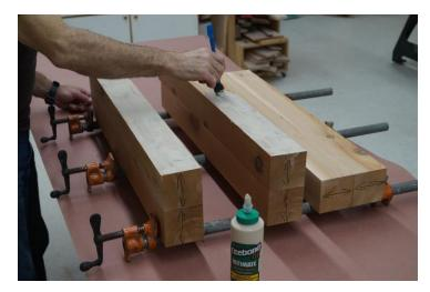
Apply glue to the remaining edges of each sub-assembly.
