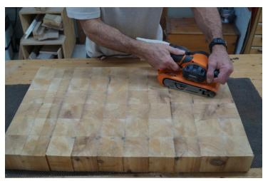
After the glue is dry, sand the faces flat. I used an 80grit belt on a belt sander. You don't need to get the faces table top smooth, just level out the highs and lows.
