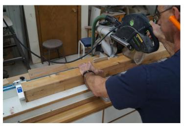
With the squared end against a stop block, cut the posts to 31-1/2". If you don't have a miter saw you can use a circular saw (making two passes) or handsaw. But keep the cuts square, or you'll spend lots of time sanding later.
