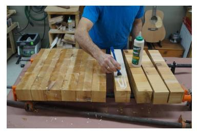
Apply glue to the long grain faces, then rotate the pieces so the end grain is up.
