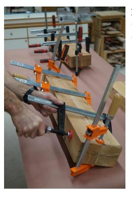
Next, apply clamps across the glue joint. Clean excess glue off the surface with a damp rag, and allow the glue to dry.
