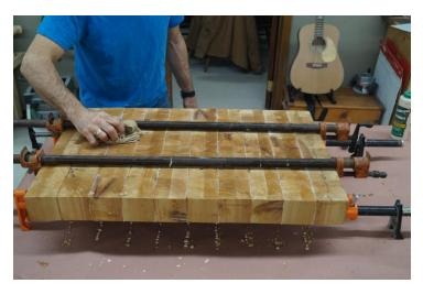
Clamp with four clamps; two above and two below. This will help the slab stay flat. Wipe off excess glue with a damp rag. Allow the glue to dry.
