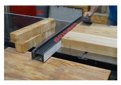
Make a cut from one face with the end grain riding against the table saw fence.
