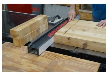
Flip the slab over, and make another cut to complete the crosscut.
