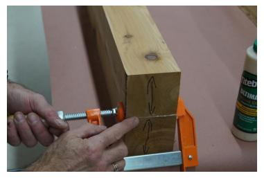
With the boards stacked, position a clamp so it bridges the seam. This helps keep the faces aligned.
