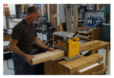
Plane both faces of each subassembly. Remove enough material to make the surfaces flat. Be sure you plane all three subassemblies to the same thickness.
