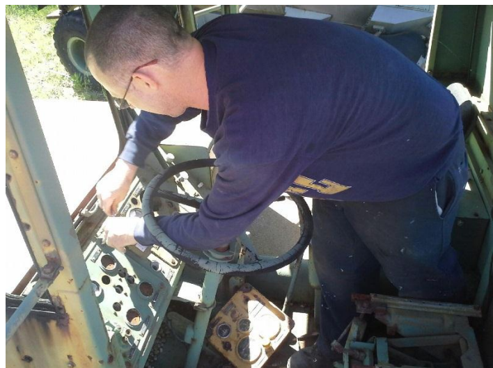
Museum volunteer John Griffin, replaces the instrument panel on the 290M. John had to assemble components from three different instrument panels to make one good panel.
