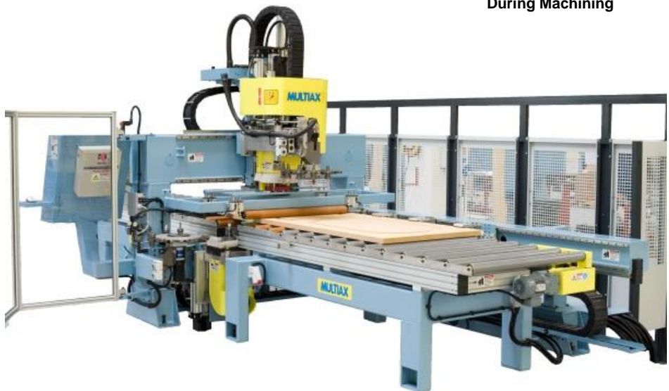
Pinch Rollers on the Top and Bottom Stabilize the Panel During Machining
