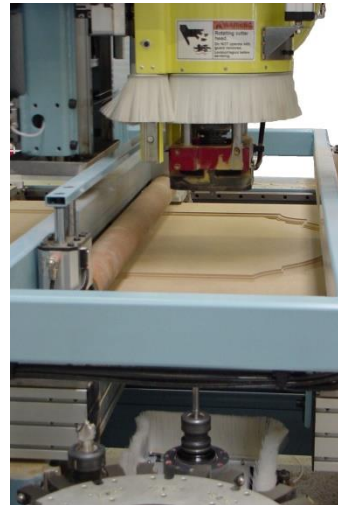
One or Two Top Spindles One or Two Bottom Spindles With or Without Tool Change and Independent Movement
