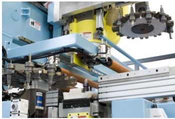
Automatic Tool Changer with Rack for 4 Tools or turn table for 8, 12 or 16 Tools
