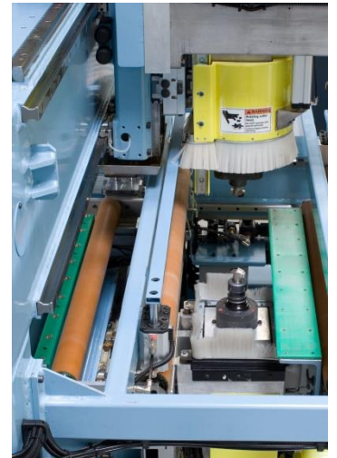
One or Two Top Spindles One or Two Bottom Spindles With or Without Tool Change and Independent Movement
