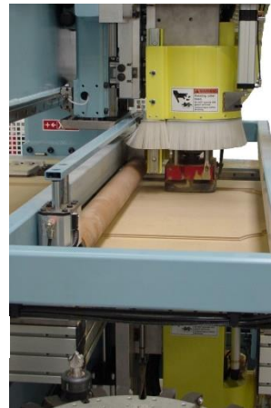
Optional Integrated Floating on the Top Spindle Motor
