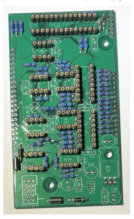
Install the fourteen 100nf COG capacitors C1, C2, C4, C5, C6, C7, C8, C9, C11, C12, C13, C14, C15 and C17. Also install the LD1117V33 voltage regulator.
