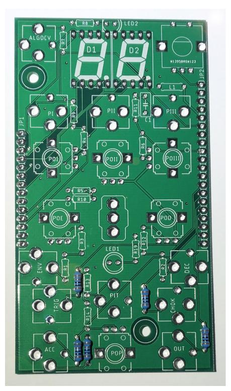
Install and solder the six 100K resistors R3, R4, R5, R6, R12 and R14
