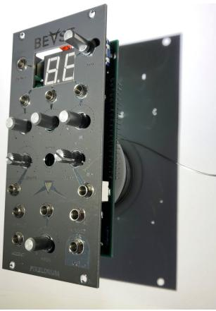
Carefully place a washer and nut on the PI and PIII pots. Also place two knurled jack nuts on the accent and out jacks. Very gently tighten the nuts until they are "finger tight" DO NOT over tighten them as they will twist the pots and jacks and/or pins will be bent.
