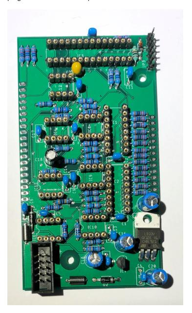
Cut the female pin headers to size, install on the opposite side of the board and solder one pin on each header. Now connect the brain board to the IO board.
