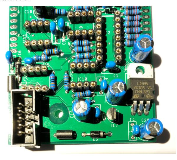
Cut a 1x6 piece of male pin header and install it into JP3 – this can be used to connect a PicKit3 programmer for firmware updates.
