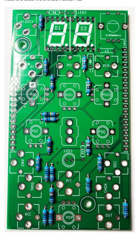
Install and solder the two 220 ohm resistors R8 and R19
