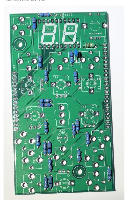
Install and solder the two seven segment displays  ${\rm D1}$  and  ${\rm D2}$
