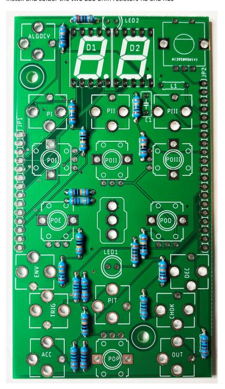
Install and solder C1 and L1
