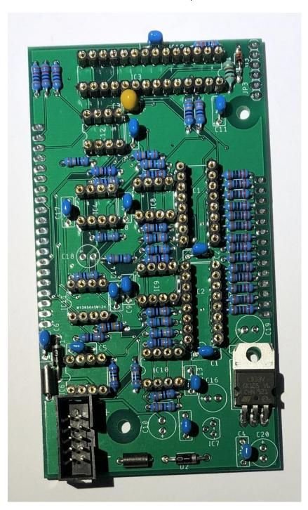
Install the one 1uF non polarized electrolytic capacitor C18 and the four 100uF electrolytic capacitors C10, C16, C19 and C20 paying attention to polarity – the longer lead is positive lead, the shorter lead pointed to by the arrow is the negative lead.
