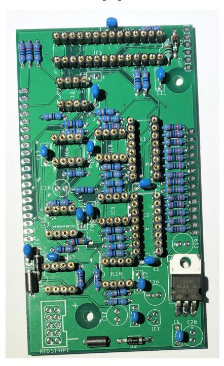
Install the 10 PIN IDC Eurorack power header, making sure the header key/"cut-out" is oriented facing the right hand side of the board as per the photo below.
