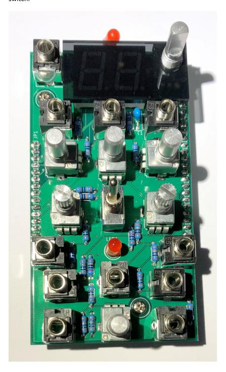
Place the panel back on. Place the nut for the SPDT switch on and finger tighten.
