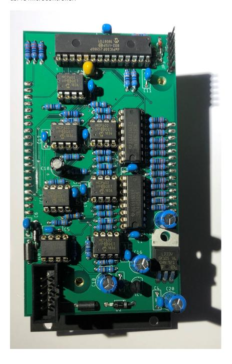
Separate the IO and brain boards. Double check all solder joints and look for shorts. When you are happy join the boards together and do a quick power on test. If everything appears to work, install the two screws in the brain board to the standoffs to secure the boards together. Lastly install the knobs.
