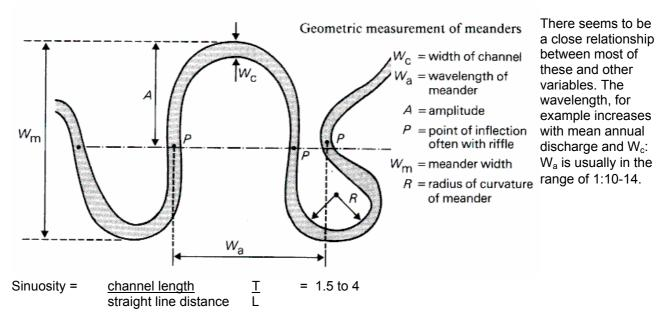
In general, pools and riffles are spaced at intervals about 5-7 times the channel width.
