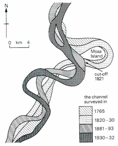
Oxbow Lakes. If the sinuosity becomes too great, a river flood may be able to break through a meander neck thereby straightening the channel, increasing its gradient and reducing energy loss. The abandoned channel, a cut-off may be used during floods but frequently they become
