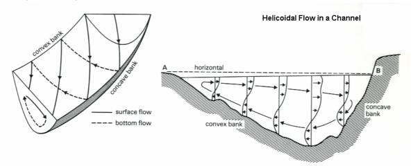
The greatest erosion of the concave slope occurs just downstream of the axis of the meander bend. This causes the meander to migrate down valley. Rates of down-valley movement of up to 15m a year in some rivers. The section of the Mississippi shown below shows a typical shifting meander pattern. The cut-off or oxbow that occurred in 1821 considerably accelerated the rate of change.
