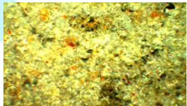
Figure 6. Optical microstructure (200X) of Electroless Ni-P nano ZnO coated sample after exposed to corrosion test
