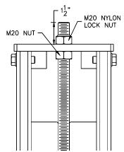
Fig 14 - Lock Ladder Assembly
