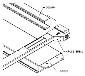
Fig 5 - Column/Cross Beam Assembly
