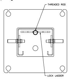
Fig 13 - Locking Ladder Orientation
