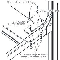
Fig 29 - Base Installation
