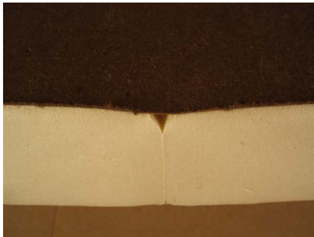
Knit line and V-groove close-up (after conditioning)
