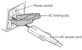
Plug the free end of the power cord into a power outlet (**D-1**).
