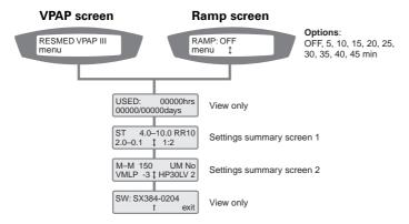
Figure 1: VPAP III ST-A Standard Menu Series
