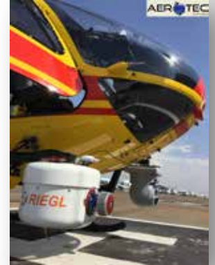
mounting example on a helicopter (EC135) for power line mapping/inspection
