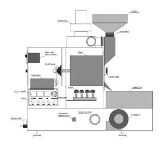
THE BC-3 MD IS A HEAVY DUTY ROASTER BUILT WITH A CARBON STEEL BODY WITH APPROVED POWDER COAT HIGH TEMPERATURE BODY IN BLACK. THE HOUSINGS COME IN MANY CHOICES. TWO EXHAUST PIPES COMES OFF THE BC-3 AT 3" AS SHOWN BELOW AND CAN BE EXHAUSTED OUT OF BUILDING SEPARATELY OR CONNECTED WITH A BLAST OR BACKDRAFT DAMPER
