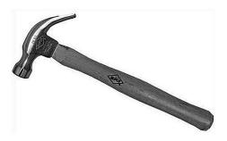
You would have to deliver a blow which is much more powerful than the hard nylon head hammer and could deform or even break the PVC extrusion (TS79W/C/B)
