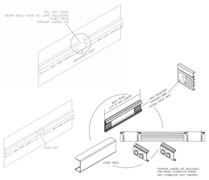
The straight jumper kits (and the elbow sections) include all the necessary parts to jump between the two backplanes. Installation of the straight jumper is similar to how the field modified elbows are installed.
