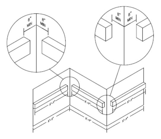
In order for the sections to fit, it will be necessary to adjust the length(s) of the interior or exterior elbow piece. The elbow pieces were designed with this situation in mind and thus can be field modified (cut) to connect the backplane sections together seamlessly.
