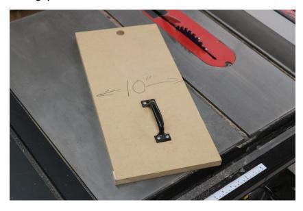
This jig works great for ripping thin strips. Keep the math simple by making the width of the jig an even number. The "foot" at the end of the jig, ¼" thick, acts as a hook to engage the material you're ripping.
