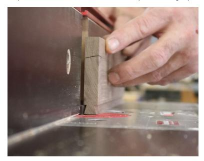
Use the same dovetail bit you used with the spline jig. Set the height of the bit so it's slightly higher than the depth of the socket. Position the fence so you're barely cutting into the face of the board. Cut from both faces.
