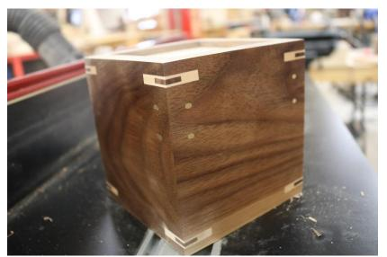
Double splines are easy to do, but require a few specific steps. In this case, a 1/4" bit was used first, the maple spline glued in, and then a 1/8" bit was used, followed by a walnut spline.
