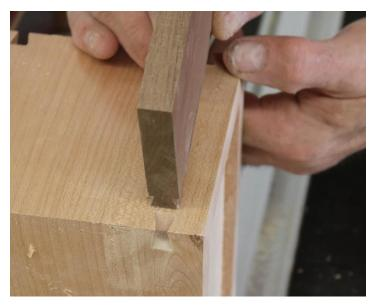
Check the size of the resulting tail against the socket. If the tail is too wide move the fence back slightly, exposing more bit, cut from both faces again, and check the result.
