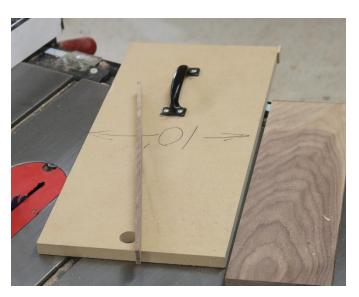
Adjust the position of the rip fence as needed to get the right size spline.
