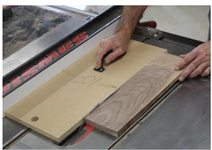
Push the sled and board past the blade together, allowing the hook on the jig to propel the board forward.
