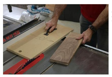
Engage the end of the material on the hook, and push the edge of the stock against the edge of the jig.
