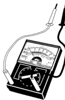
CORRECT VOLTAGE AT RECEPTACLE CHECKED WITH MULTI-METER
