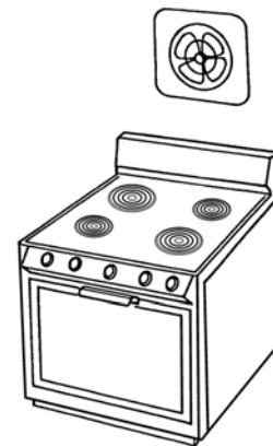
FUNCTIONAL VENTILATION REQUIRED (FAN OR PASSIVE VENT) IN MOBILE HOME COOKING AREA (GAS OR ELECTRIC)
