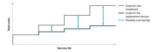
With the replacement service, the total costs of the diaphragm seal system can be clearly lowered. In this way, the service life of the process transmitters can be fully utilized and only the diaphragm seal and the assembly parts needs replacement, preventatively or after failure.
