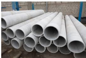
Asbestos Cement Pipe
