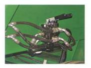
Conveniently located drum rotation and downrigger/cart controls.
