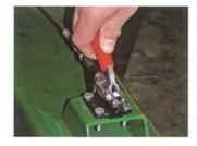
Positioning lock for turntable is conveniently located on the draw bar.
