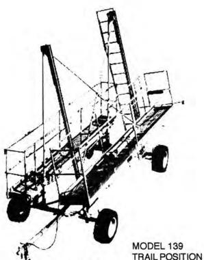
Shown above is an example of a Model 139 in trail position for highway tow. the example consists of a Model 139 with optional wide tires, 2" Ball hitch, 1 Intermediate Level, and a Light Bar. To tow, in Trail Position, adjusting arm threads must be screwed completely in to give a clearance of approximately 13 ft. 5 in.
