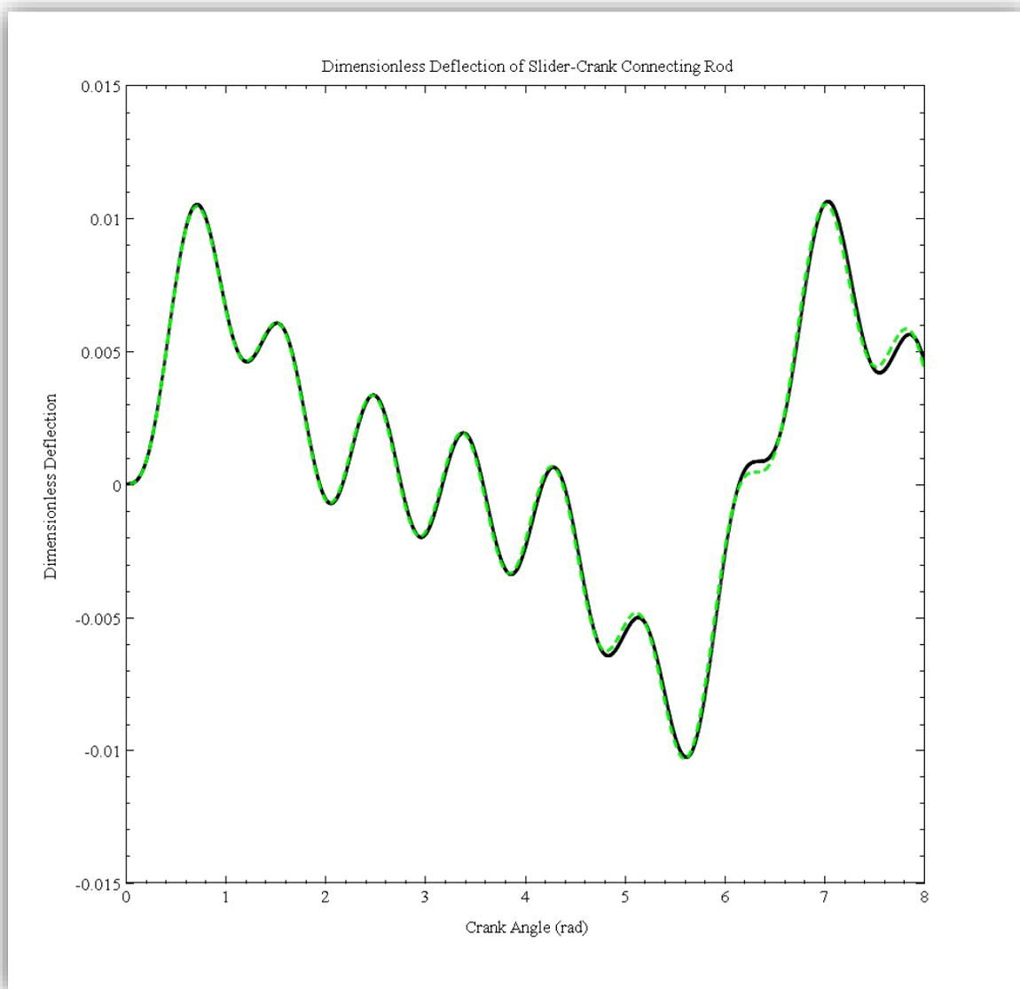
**Figure 6.** Dimensionless deflection of the middle-node of the two-element discretization of the connecting rod (GREEN). The semi-analytical solution provided by (Chu and Pan, 1975) is given for validation (BLACK).
