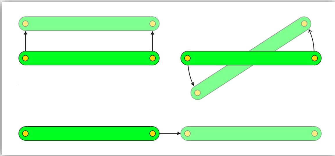
**Figure 2.** Rigid Body Modes of the Connecting Rod.
