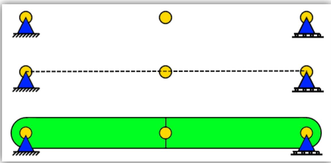
**Figure 1.** The design process of a discretized deformable body. First, the nodal locations as well as the reference conditions are specified (TOP). The next step is to specify the element connectivity, or which nodes make up each element (MIDDLE). Finally, the element geometric and inertial properties are specified in order to fully define the deformable body (BOTTOM).
