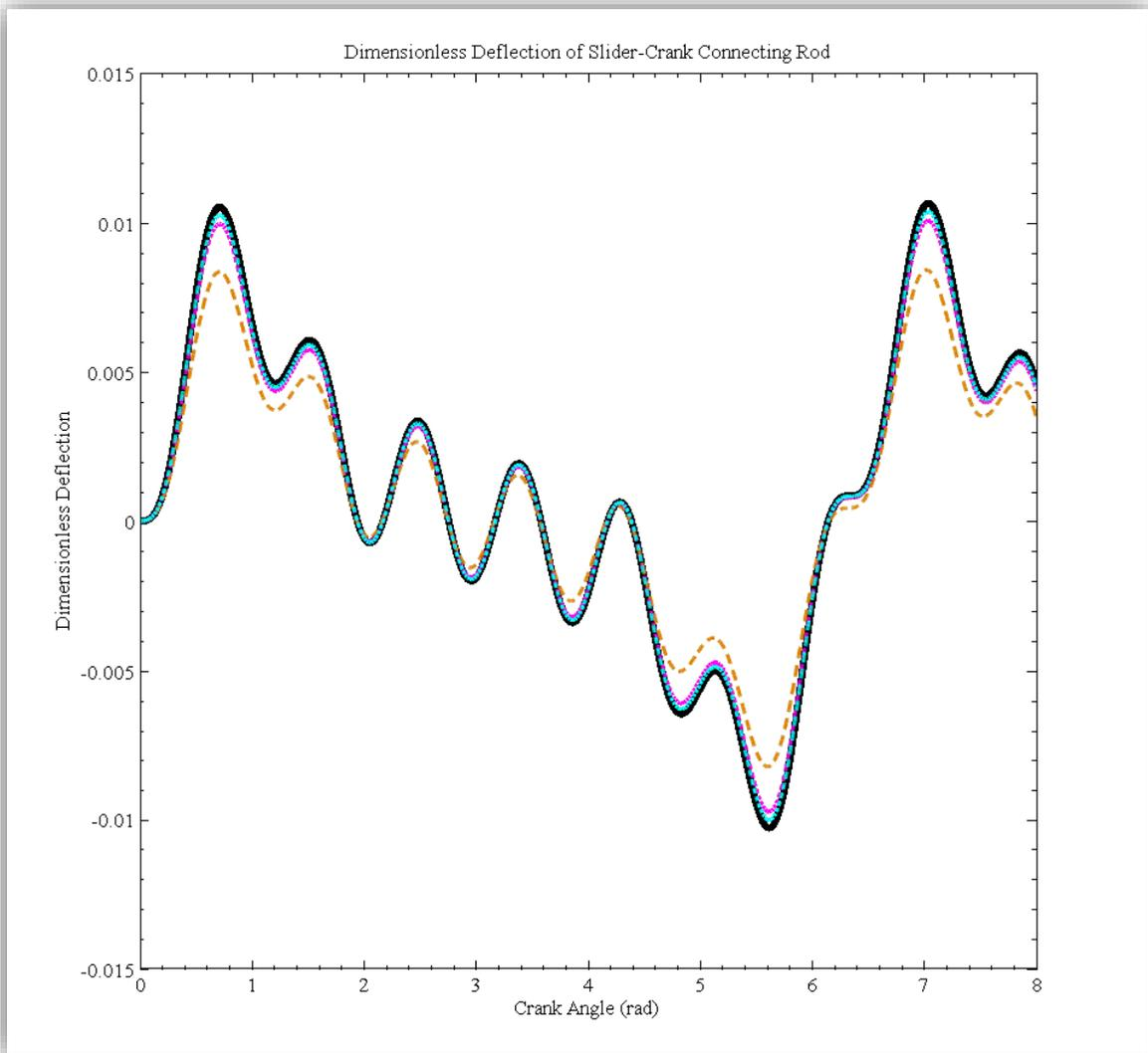
**Figure 5.** Dimensionless deflection of the middle node of the connecting rod for two-element (ORANGE), four-element (MAGENTA), and six-element (CYAN) discretization. A semi-analytical provided by (Chu and Pan, 1975) is shown for validation (BLACK).
