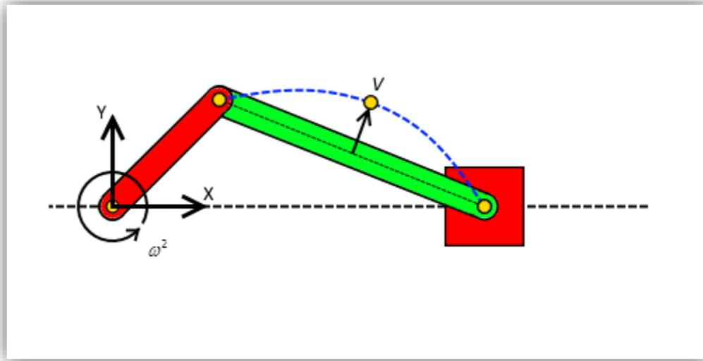
**Figure 4.** Slider-crank mechanism
