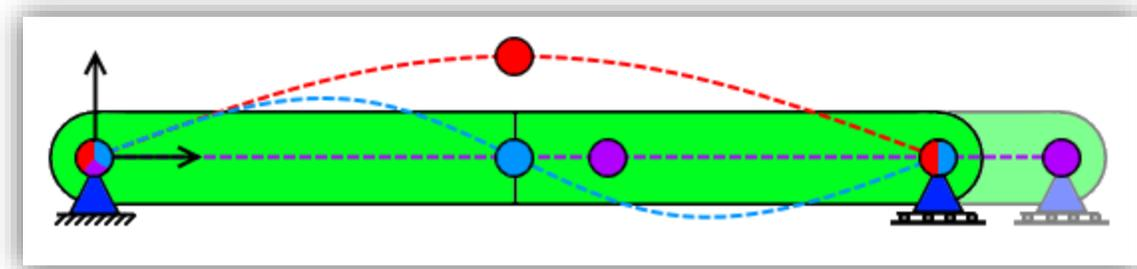
**Figure 3.** Examples of the connecting rod modes of deformation, using simply-supported reference conditions. Two bending modes (RED/BLUE) and one axial mode (PURPLE).
