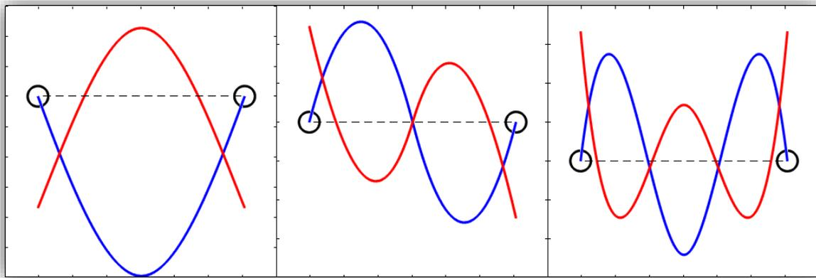
**Figure 7.** First three modes of deformation for the connecting rod, discretized into two elements, for simply-supported (BLUE) and free-free (RED) reference conditions.
