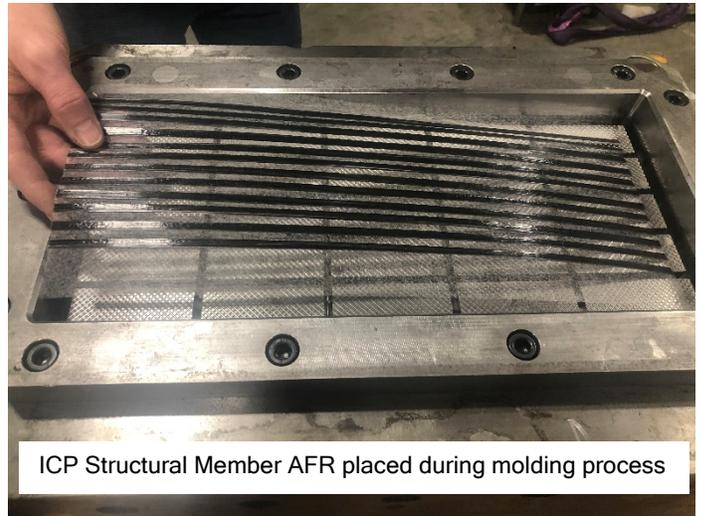
ICP Structural Member AFR placed during molding process
