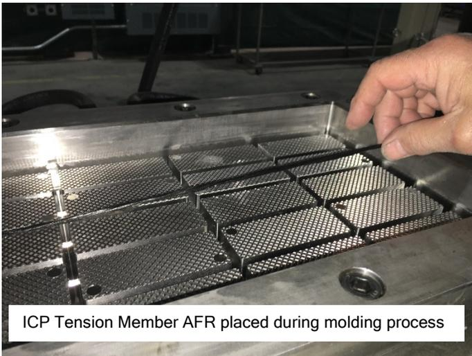
ICP Tension Member AFR placed during molding process
