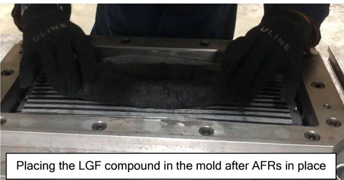
Placing the LGF compound in the mold after AFRs in place
