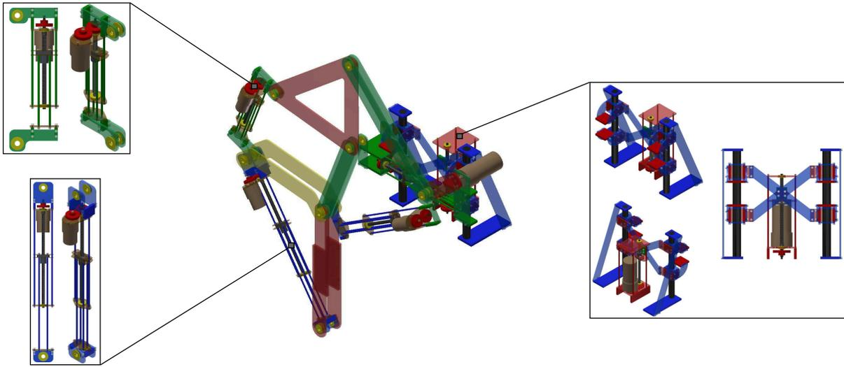
Fig. 5. A fully-functional reconfigurable Jansen leg with four actuators suitable for the transformation procedure presented in section IV (“single link” column) (**center**). Zoomed areas present details of the grounded system (**right**) and some of the links of variable dimension (**left**).
