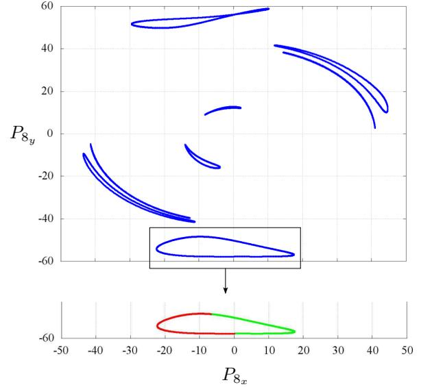
Fig. 3. **Top:** Possible locations of point  $P_8$ , the foot, in all assembly modes of a standard Jansen leg. The lowest sampled curve corresponds to the trajectory used in walking platforms. **Bottom:** Traced foot trajectory of a standard Jansen leg. The green path corresponds to the assembly mode family given by  $A_{1,2,3} > 0$ ,  $A_{1,3,4} > 0$ ,  $A_{1,3,6} < 0$ , and  $A_{6,5,7} < 0$ . In the red path,  $A_{1,2,3} < 0$ ,  $A_{1,3,4} > 0$ ,  $A_{1,3,6} < 0$ , and  $A_{6,5,7} < 0$ .
