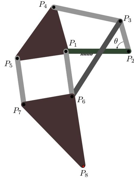
Fig. 2. The Jansen leg, a one-mobility planar linkage of eight links and three independent loops.
