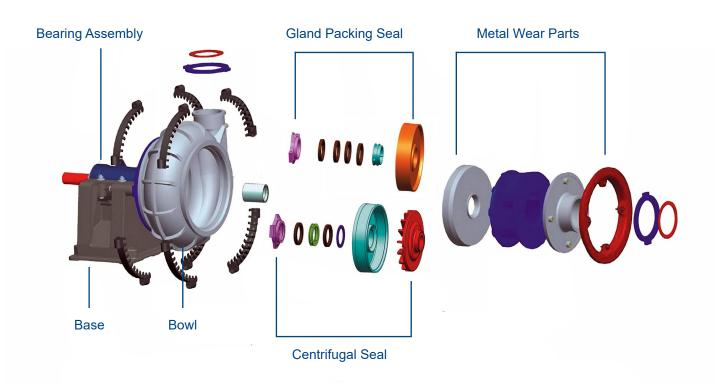
Multi-options of sealing and bearing assembly for one model Gravel pump. Bowl,Impeller,Throatbush,Frame Plate Liner are made by ultra chrome alloy.
