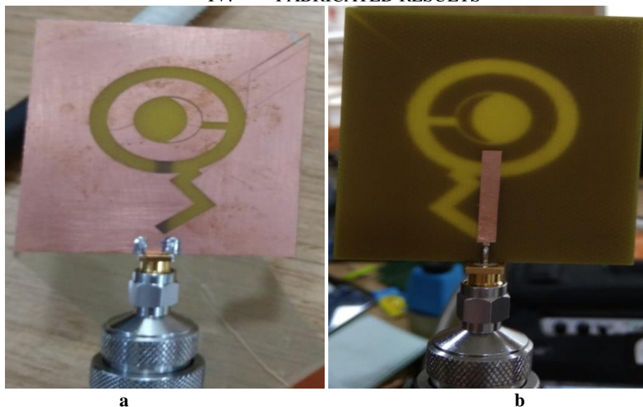
Fig.6: (a): Proposed Antenna Front View (b): Back View
