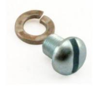
The problem is that the ignition cam screw may not hold the cam down tightly to the distributor shaft. After a bit of driving, the cam rotates into a more and more "retarded" position and the engine loses power.
