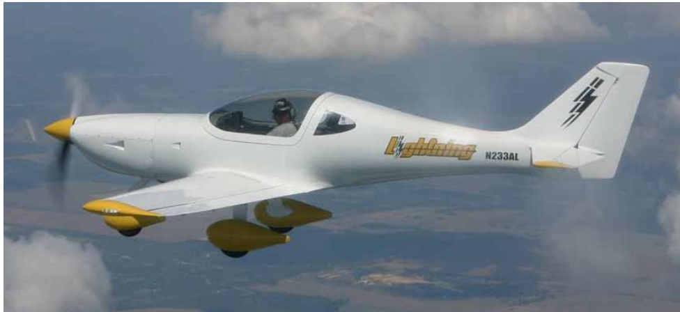
The prototype Lightning, designed around the 120 HP Jabiru 3300.
