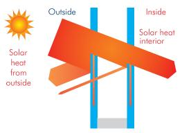
Solar heat is reflected, absorbed and transmitted
