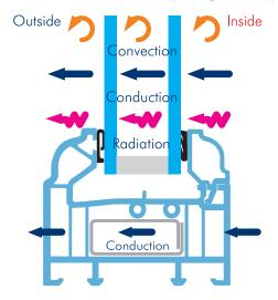
Thermal losses from convection, conduction and radiation
