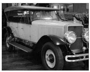
1924 Doble steam car, Perhaps the most advanced steam car ever built, it could raise steam in 90 seconds from a cold start and cruise all day at 70 mph. Top speed was 100 mph. Fewer than 45 cars were built.
