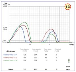
A special software function allows the average of the displayed values to be calculated and the three overlaid graphs to be viewed in detail (fig. **13**).
