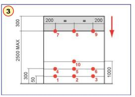
There are thirty measurements necessary, three for each measuring point.
