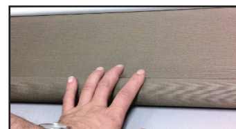
4. Attach fabric to tube and roll up
