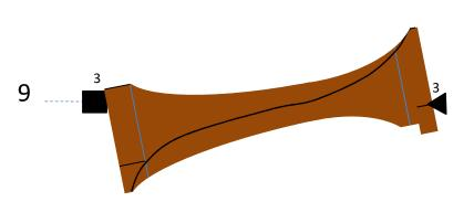
Move to Axis 2. Repeat the same cuts. This time, try to make the cut line meet up with the cut line from Axis 1. It should be a single line created between the two curves, with no flat spots. You may find that you need to return to Axis 1 to cut a little deeper, but you can also do that after doing axis 3.
