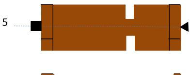
Use a parting tool to cut into the lowest point. About 5/8" or a little more works well.
