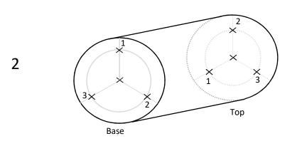
On the base, mark the center and 3 equilateral points and label them. On the top, repeat the same four marks, but make them a little closer to center. The distances from center can be changed to your liking. Be consistent when making duplicates. The marks on the top should be rotated one position, such that 1 is opposite 2, 2 is opposite 3 and 3 is opposite 1. The direction of the rotation will be the direction of the twist.
