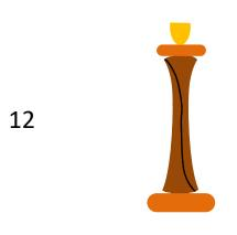
Cut a top and bottom for the candlestick. A contrasting color will look better, with the bottom being larger than the top. You can put a brass or other metal cup on the top, or you can cut the cup out of wood. If using a wood cup, I suggest using a brass insert around the rim to insure the candlestick won't burn or char if the candle is left unattended. I have found a ¾" hole makes a good fit for a taper candle. Some references say 7/8", but that makes for a loose fit.
