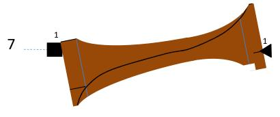
Put the piece on axis 1. Turn away only about 1/16" of the original curve. Stop frequently and try to make sure no part of the cut exceeds 1/3<sup>rd</sup> of the original shape. Use the marks on the side to judge what 1/3 of the circle is. The line created between the first cut and the second should be smooth and flowing. Any bumps will put a curve in the line.
