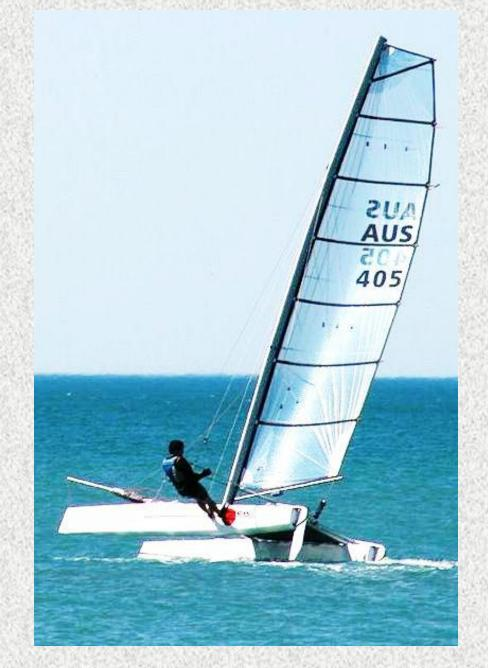
Using The Sailor's Body As An Additional Counterweight for ROLL stability!
