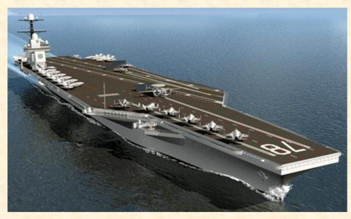
The shape of the hull ensures 97,000 tons of water is displaced while the water level on the outside of the hull is well below any dangerous line
