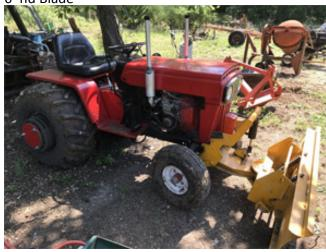
Farm King garden tractor, 16 Eaton hydrostatic, 20 hp Honda, w/4' blade
