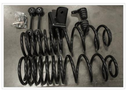
Here's the Deluxe 2/4-drop kit from McGaughys. The front is relatively straight forward as the new spindles raise the wheel hub for the drop. For the rear, a set of springs will provide a 4-inch drop. Since the drop changes the position of the rearend, new rear sway bar end links, bump stops and a track bar relocating bracket are included as well.
