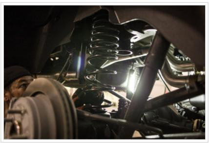
The new rear coils have a different spring rate that allows them to compress more to lower the truck. They are placed in easily just like the stock versions and lock into place by raising the rearend.
