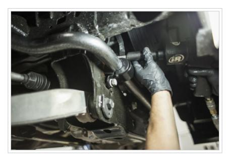
The heavy-duty Hellwig sway bar can be attached the same way as the factory version.
