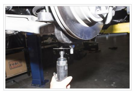
On the lower side, the spindle is secured to the ball joint using the supplied nut. Because the wheels are essentially being raised up in relation to the suspension, the excess threads must be cut off to fit the stock wheels. Even if you're running large wheels, you might want to do this anyway so that you can use your 17-inch spare if you blow a front tire. After the brakes are on, the front is finished and the wheels can be reinstalled.
