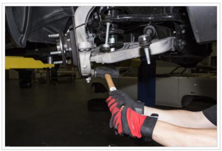
If your ball joints are worn out and need replacing, use a pickle fork and air hammer to remove them. Typically this will damage the boots, so if you plan to reuse them, strike the spindle with a hammer perpendicular to the ball joint. It may take a few whacks, but it will eventually pop out.
