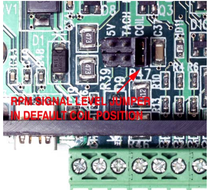
Figure 13 – RPM Signal Level Jumper
