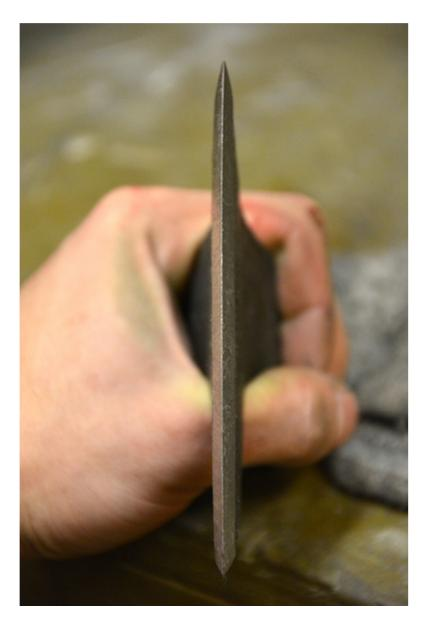
With the 80 grit belt I grind the edge down to a burr. Once you can clearly see the burr on both edges I progress to the 120 grit belt. From here it's rather simple... Once you change grits you need to remove the previous grit marks, and create a burr. After the burr is made go up a grit until you reach your highest grit.
