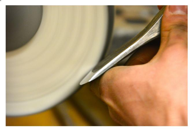
I finish grinding with the 36 grit belt when the edge of the axe reaches approximately 10 thousandths of an inch as pictured above. Now I move onto my 80 grit belt and remove all the 36 grit marks.
