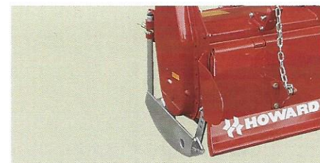
Depth control skids.
