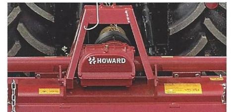
Selectatilt four speed gearbox.
