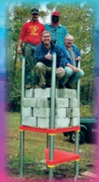
Molded Deck Tested to Over 3,000 lbs.
