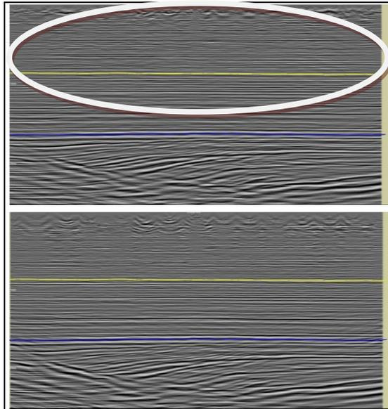
Figure 2: Top: PSTM5D. Bottom: PSTM. The obvious improvement of PSTM5D is the continuity in the shallow to mid-section as indicated by the white circle. Yellow and blue are the horizons picked for qc purposes.
