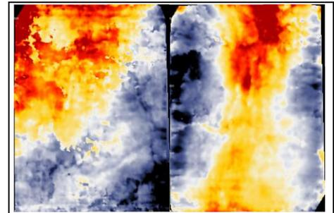
Figure 3: Time structure maps. Left: Yellow horizon. Right: Blue horizon. The yellow horizon shows a more stratigraphic structure while the blue horizon shows a north-south faulted anticlinal structure. High: Pink/red color. Low: grey/white color.
