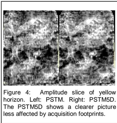
Figure 4: Amplitude slice of yellow horizon. Left: PSTM. Right: PSTM5D. The PSTM5D shows a clearer picture less affected by acquisition footprints.
