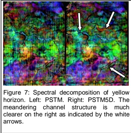
Figure 7: Spectral decomposition of yellow horizon. Left: PSTM. Right: PSTM5D. The meandering channel structure is much clearer on the right as indicated by the white arrows.
