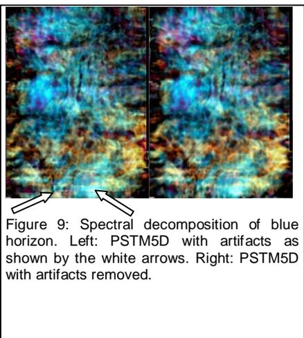
Figure 9: Spectral decomposition of blue horizon. Left: PSTM5D with artifacts as shown by the white arrows. Right: PSTM5D with artifacts removed.
