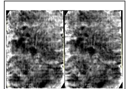
Figure 5: Amplitude slice of blue horizon. Left: PSTM. Right: PSTM5D. The PSTM5D shows a clearer picture.
