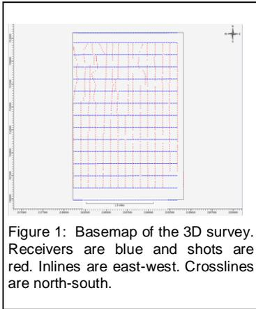
Figure 1: Basemap of the 3D survey. Receivers are blue and shots are red. Inlines are east-west. Crosslines are north-south.
