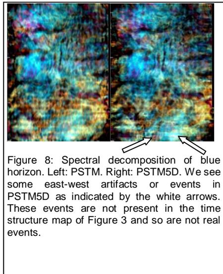
Figure 8: Spectral decomposition of blue horizon. Left: PSTM. Right: PSTM5D. We see some east-west artifacts or events in PSTM5D as indicated by the white arrows. These events are not present in the time structure map of Figure 3 and so are not real events.
