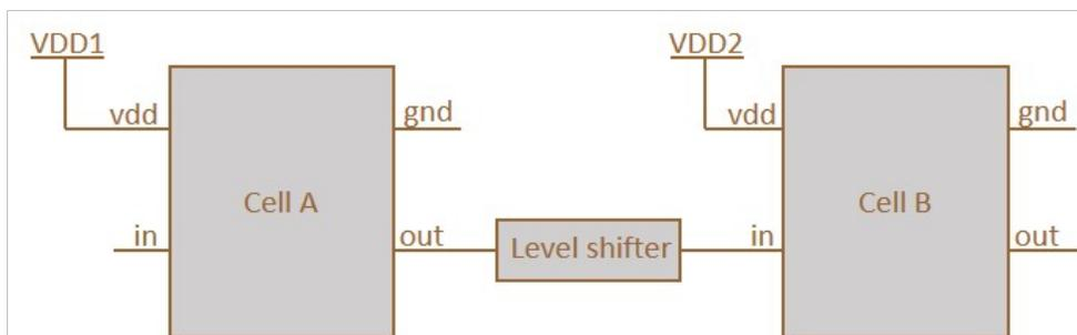
**Figure 2: Level shifter circuit connected between signal nets of two different power domains.**
