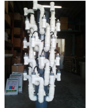
Multiple FB-50 aerator/water circulator
