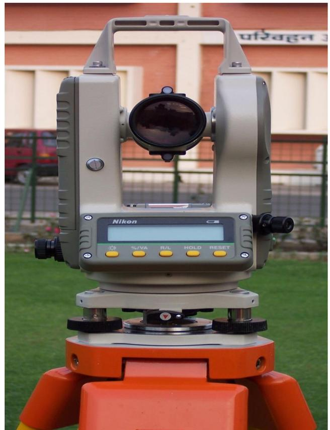
(ii) **Total Station** - This is an electronic instrument. In this instrument, all the parameters required to be observed during surveying can be obtained. The value of observation gets displayed in a viewing panel. The precision of this type of instrument varies in the order of 0.1" to 10".
