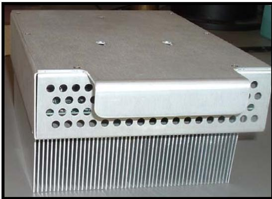
Figure 11 - 1725 Watt PA Module
