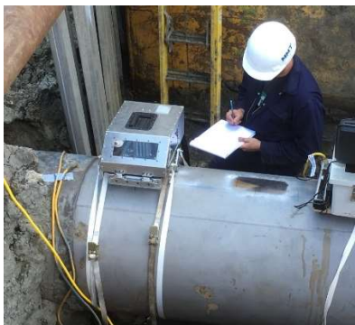
Field technician prepares surface and mounts HSD Tester to pipe.
