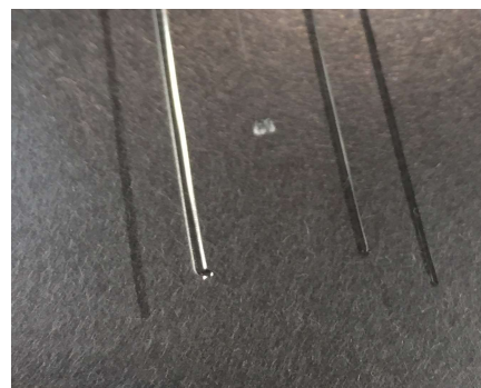
HSD Tester makes grooves and measures profiles, generating tensile properties, weld type, steel grade, and other mechanical properties.
