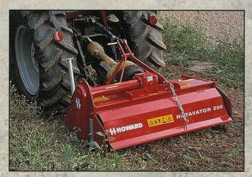
Chain side drive, equipped with a 1 in. (2.5 cm) chain.
