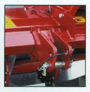
Lower brackets movable for tractors with cat. 1 and 2 linkage.
