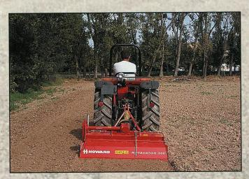
The R300B is equipped with a chain side drive. The long trailing board provides a very smooth finish.
