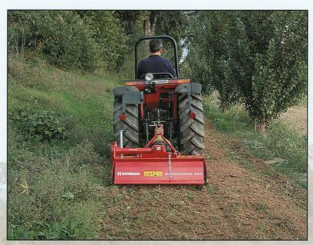
Rotavator 200-105. Specially designed for compact tractors.
