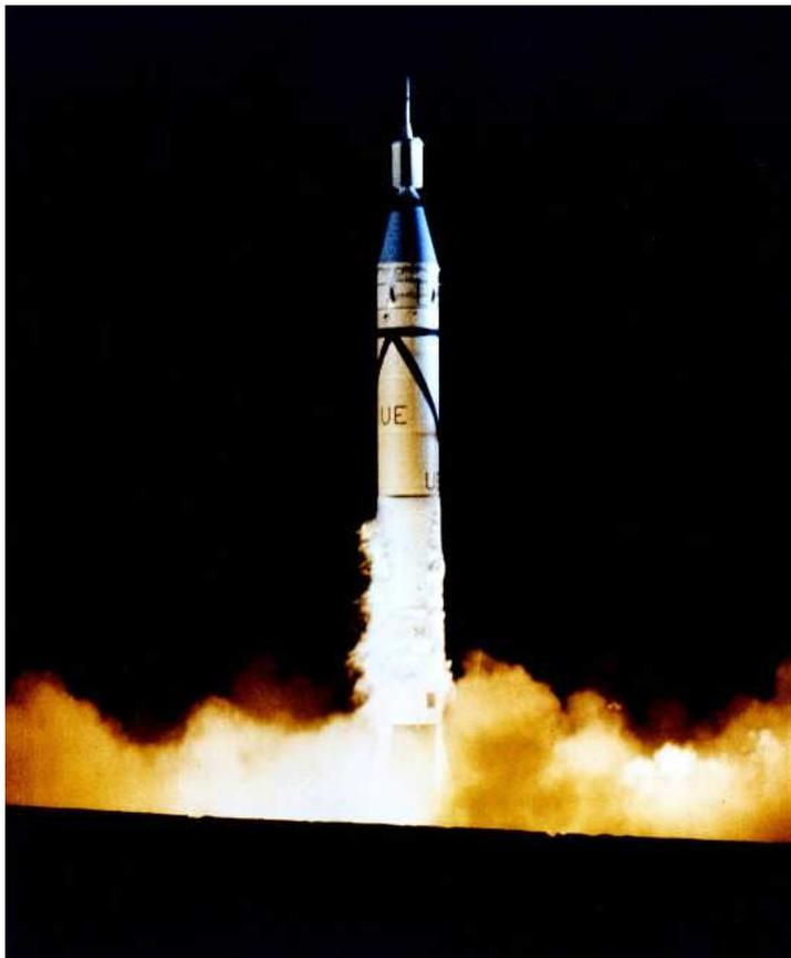
*Explorer 1 is the small section on top of the large Jupiter-C rocket that blasted it into orbit. With the launch of Explorer 1, the United States officially entered the space age. Image credit: NASA.*
