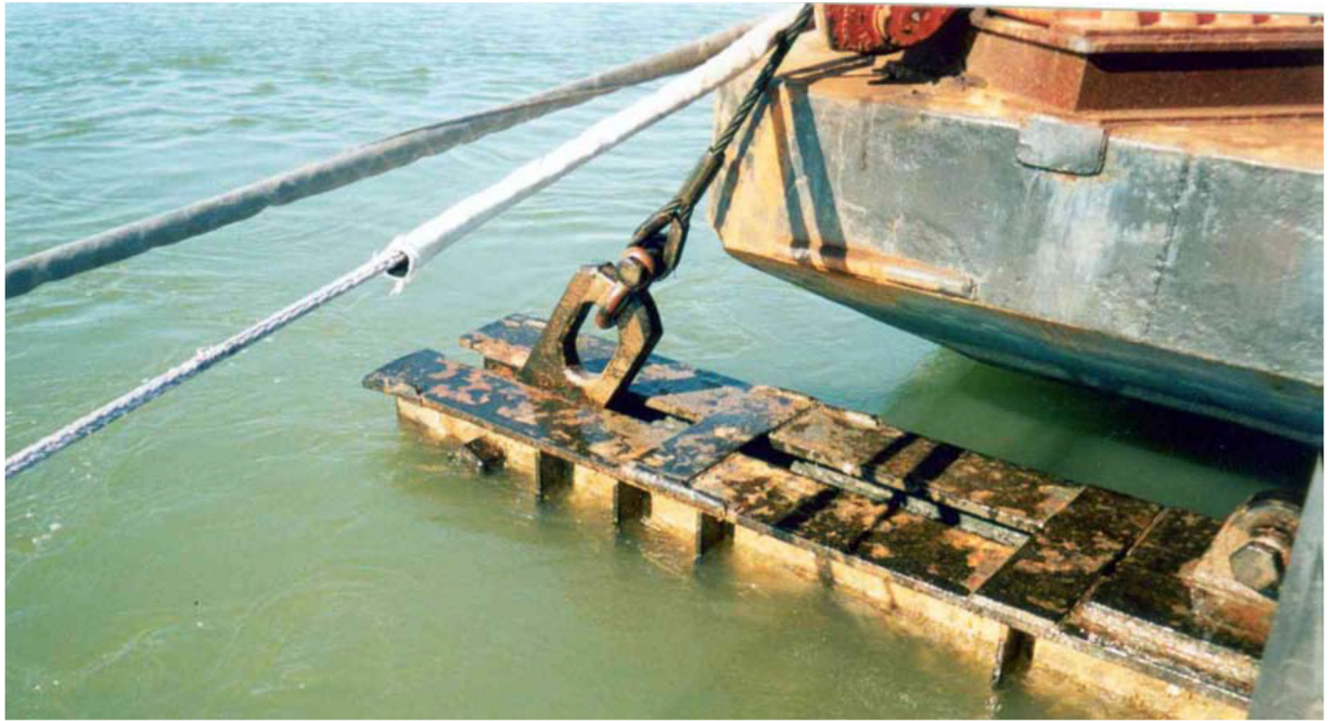
Figure 3-3 Knockdown Dredging Configuration – I-Beam Mounted on Boat Stern
