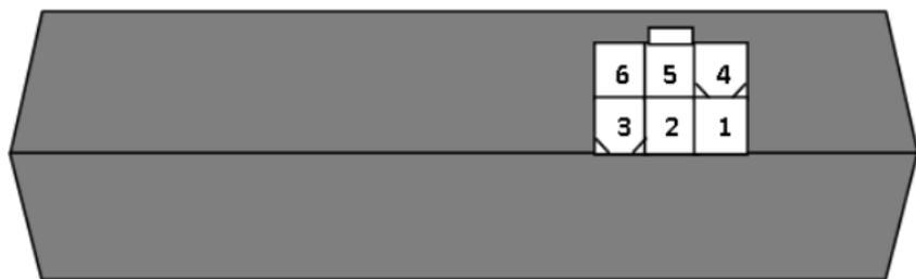
The radio interface connector on the **TurboTuner-2** is Molex part # 39-29-1068.
